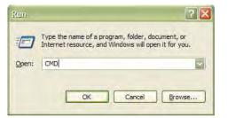
Using a PC that is connected to the same Router / Access Point as the DVR unit, bring up a Command Prompt by clicking the Start Button - Run. In the Run window, Type in CMD and click OK.
