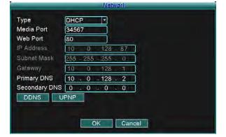
Determine the IP address shown. This is your DVR's IP address. Make a note of this.
