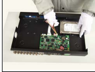
5. Install SATA power cables
