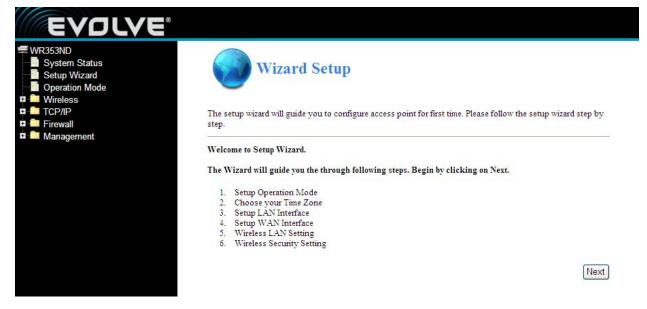
The router supports three modes: gateway, bridge, wireless ISP. You can setup different modes to LAN and WLAN interface for NAT and bridging function.
