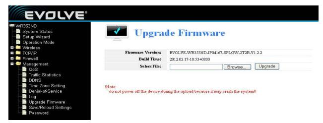
This page allows you upgrade the Access Point firmware to new version. Please note, do not power off the device during the upload because it may crash the system
