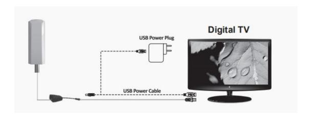
Connect the signal cable from the antenna to the signal input Jack of the power supply, connect the power supply output jack to the TV, plug the power adapter with the power supply and connect to power socket.
