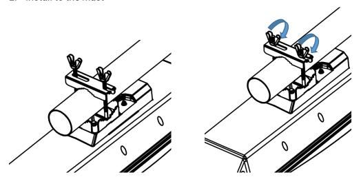
Place U-bolt through the mast, adjust the antenna bracket and fasten screws.
