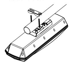
Insert the U-bolt into the hole of antenna bracket and then install the clamp in the U-bolt.
