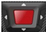
Navigate up or down, left or right in the menu. The quick access functions which can be freely assigned are on the start screen. Central button is for confirmation or enter menu.
